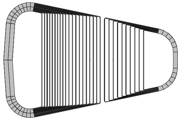
Figure 4. Conceptual sketch of superconducting trim coils. Three sets of trim coils are wound in three radial regions.
