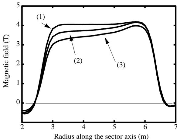
Figure 6. Field distribution along the sector axis for (1) 150 MeV/ nucleon  $^{238}\text{U}^{58+}$  ions, (2) 300 MeV/nucleon  $^{84}\text{Kr}^{30+}$  and (3) 400 MeV/nucleon  $^{16}\text{O}^{7+}$ .
