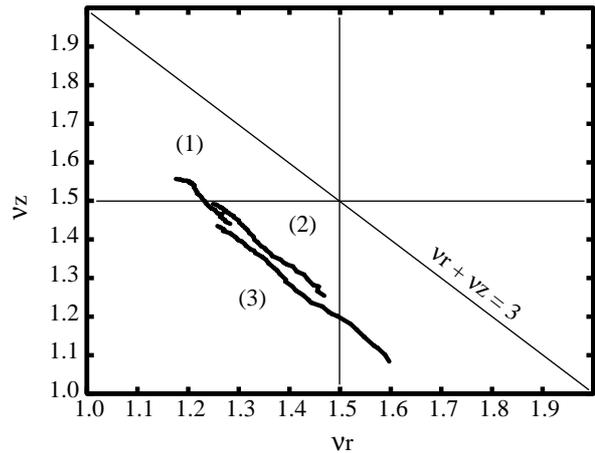
Figure 7. Tune values for typical ions for (1) 150 MeV/nucleon  $^{238}\text{U}^{58+}$ , (2) 300 MeV/nucleon  $^{84}\text{Kr}^{30+}$  and (3) 400 MeV/nucleon  $^{16}\text{O}^{7+}$ .
