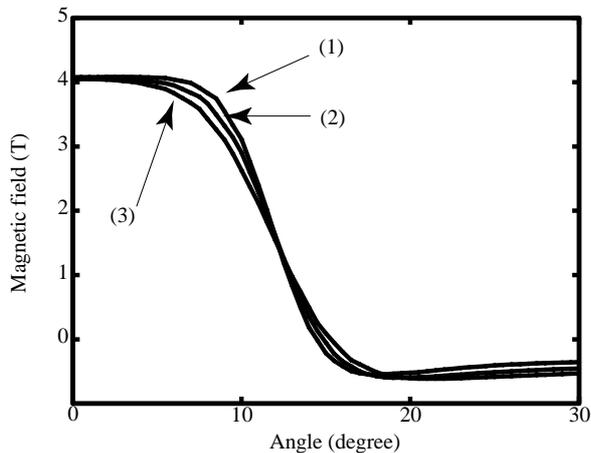
Figure 5. Field distribution along the azimuthal direction at (1)  $r = 3.58$  m, (2)  $r = 4.3$  m and (3)  $r = 5.1$  m for 150 MeV/nucleon  $^{238}\text{U}^{58+}$  ions.
