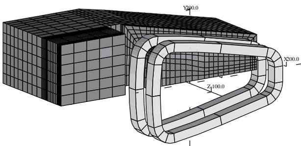
Figure 3. Example of modeled magnet for TOSCA.
