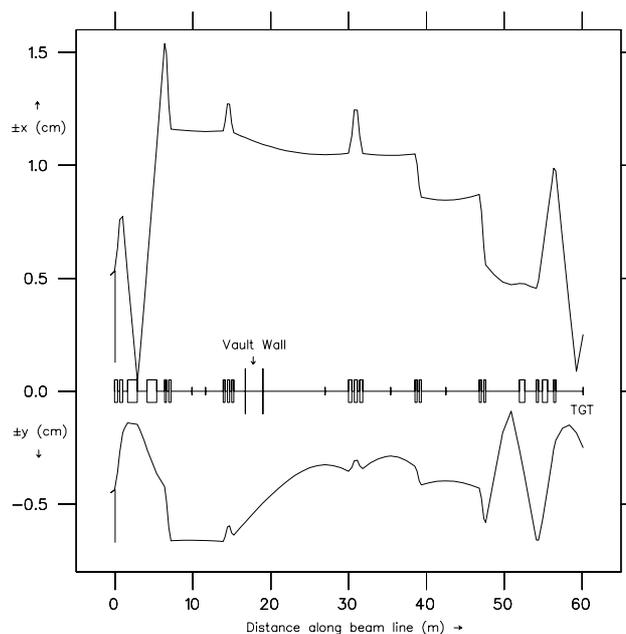
Figure 3: 500 MeV beam envelope on beam line 2A.
