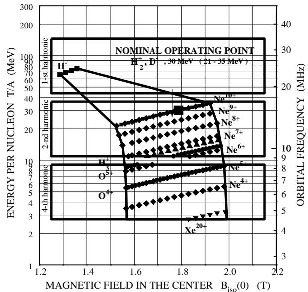
Figure 6. Operating range of the VINCY Cyclotron in terms of selected ion beams
