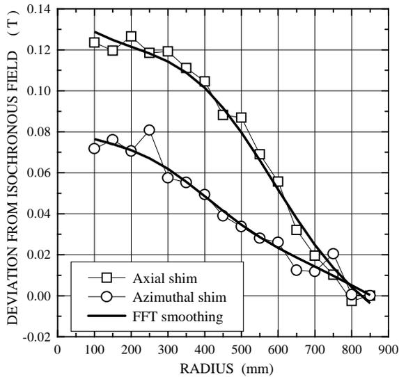
Figure 2. Deviation from isochronous field according to model magnet measurements for low level magnet excitation
