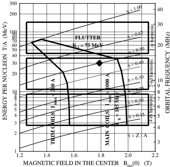
Figure 5. Operating range of the VINCY Cyclotron in terms of cyclotron parameters
