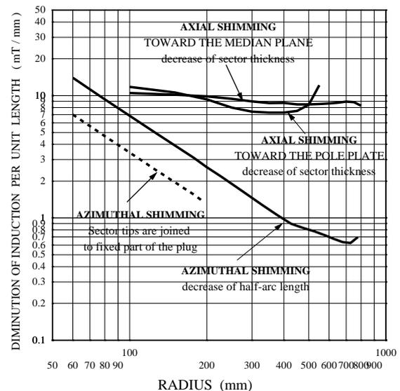
Figure 4. Sensitivity of magnetic field as a function of sector dimensions
