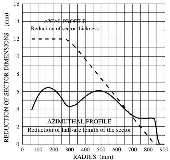
Figure 3. Axial and azimuthal profiles of the sectors
