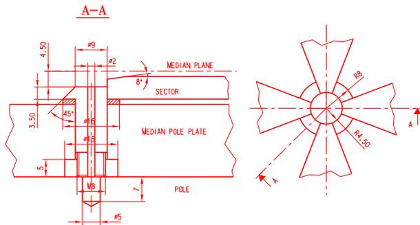
Figure 5. Final shape of the magnetic plug
