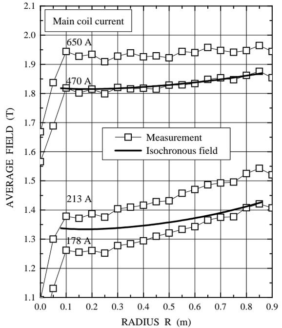
Figure 4. Radial distribution of average magnetic field in the case of azimuthal shimming
