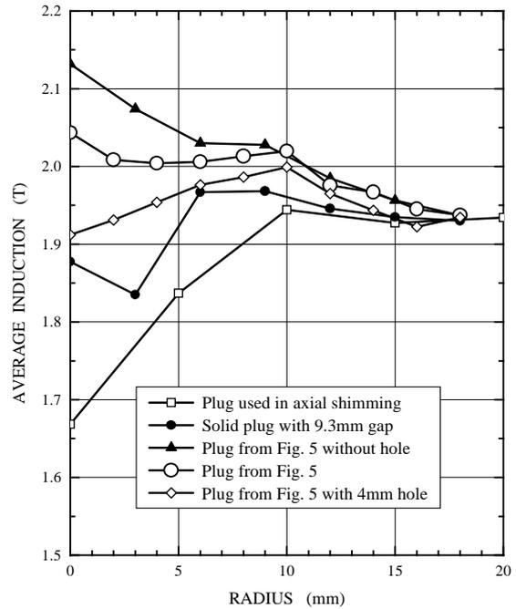
Figure 6. Radial distribution of average magnetic field for the plug shape from Figure 5
