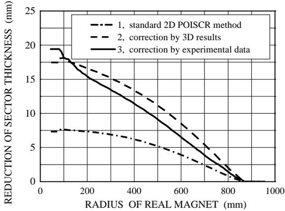
Figure 1. Three iterations in computation of the axial sector profile of the real magnet
