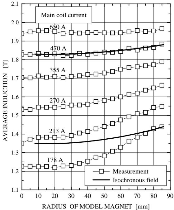
Figure 2. Radial distribution of average magnetic field for the third iteration of axial profile
