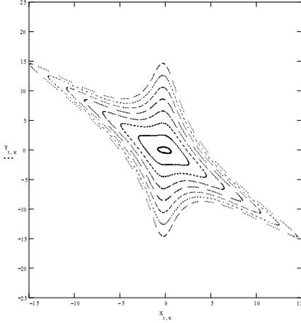
Figure 1: Phase space for “drift space plus one thin non-linear lens” map. Parameters of the kick (4) are:  $a1 = 0.2, b0 = 0, b1 = 0.45, a2 = 0.4, a0 = 1$ .
