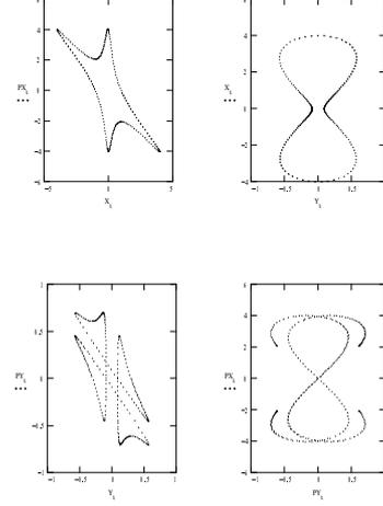
Figure 2: 2D phase space for "drift space plus one nonlinear lens" map. X-PX, Y-PY projections are on the left figures; upper right shows X-Y trajectory, lower right is PX-PY portrait. Parameters of the complex kick are:  $a = 10, b = 0.2, d = .5, h = 0, f = 1$ .
