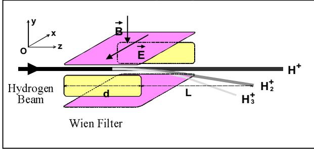
Figure 3: Schematic design of the Wien mass separator.
