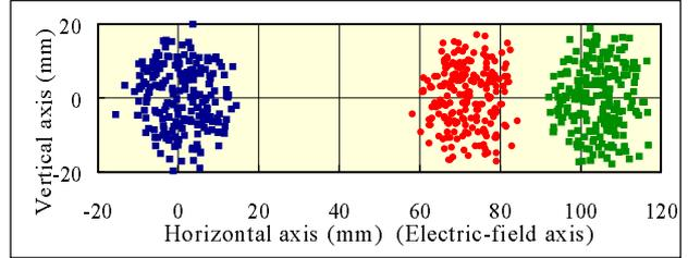
Figure 4:  $H^+$ ,  $H_2^+$  and  $H_3^+$  ion-beam distributions. They range, respectively, from left to right.
