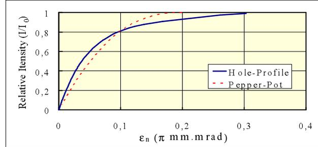
*Figure 2: Comparison of HPM and PPM intensity-emittance curves for a 500-keV, 3-mA proton beam.*
