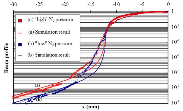
**Fig. 2** : Experimental and simulated beam profiles for two different nitrogen-gas pressures.
