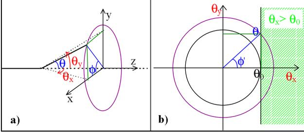
**Fig. 1** : Projection of the scattered particle trajectory onto the horizontal plane.
