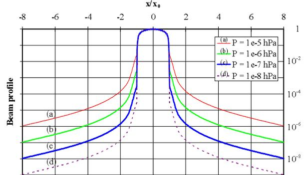
**Fig. 4** : Influence of the scattering process on the beam profile.
