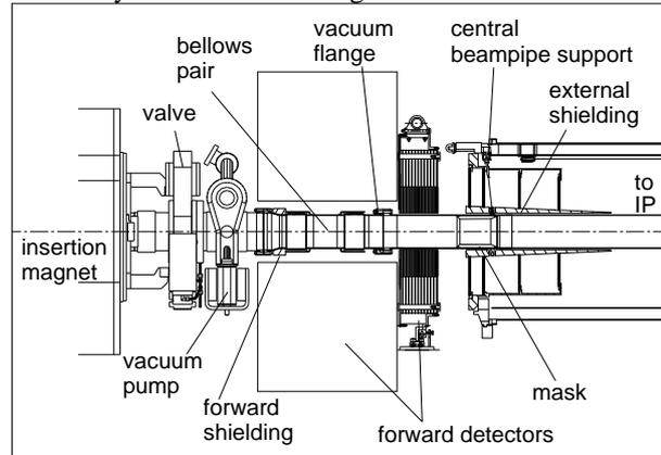
Figure 3: Detail of the ALEPH Experiment
