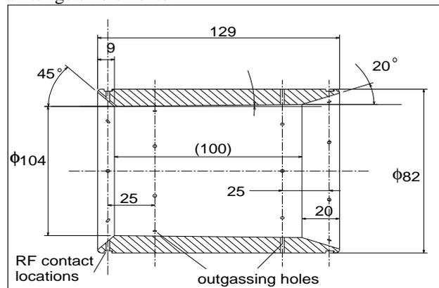
Figure 4: Section through ALEPH Mask
