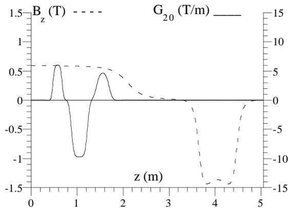
Figure 2 : KLOE IR solenoidal and quadrupolar fundamental functions.
