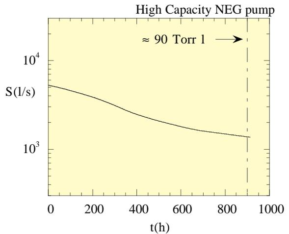
Figure 5: The result of the test on the final configuration of the DAΦNE High Capacity NEG is reported. The pumping speed  $S$  (l/s) vs. time is shown. The testing conditions relate 900 hr to  $\approx 90$  Torr l of pumped gas.
