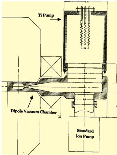
Figure 3: Final full scale prototype of DAΦNE TSP-SIP pumping station and Dipole vacuum chamber.
