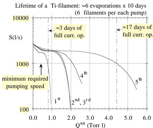
Figure 4: The pumping speed  $S$  (l/s) of the DAΦNE TSP with one Ti filament is reported vs. the total pumped gas load  $Q^{\text{tot}}$  (Torr l). Each filament allows 6 sublimation covering  $\approx 60$  days of full current operation (after conditioning). Each TSP cartridge provides 6 filaments.
