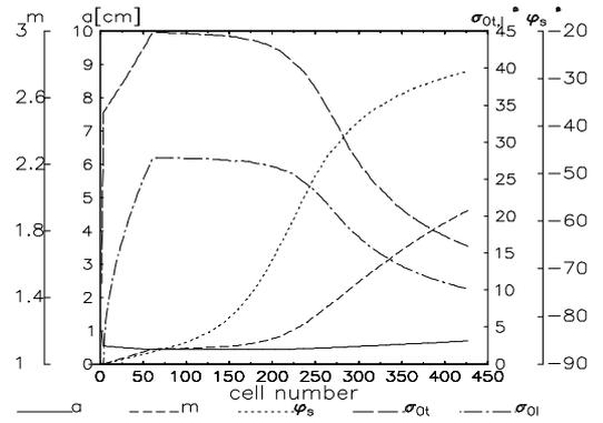
Fig. 1. Plot of the dynamics parameters of the equipartitioned  $D^+$  RFQ .
