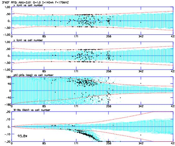
Fig. 2. Particle trajectories in the equipartitioned RFQ in case of 140mA.
