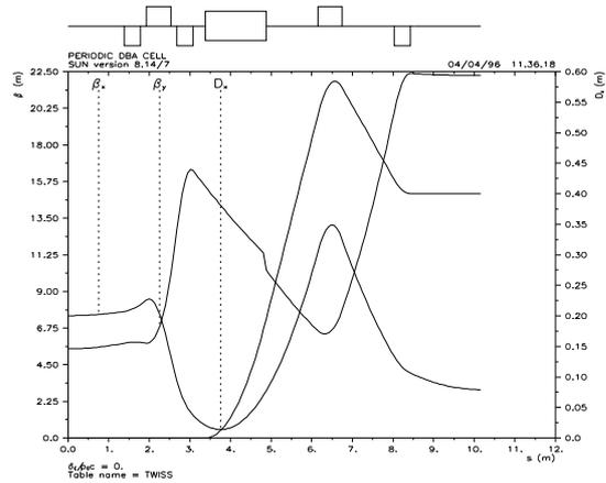
Figure 2: Lattice functions for DBA arc half cell in low emittance mode.
