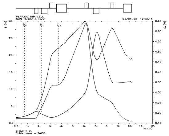
Figure 3: Lattice functions for TBA arc half cell in high emittance mode ( $\nu_x^c=5/6$ ,  $\nu_y^c=5/6$ ).
