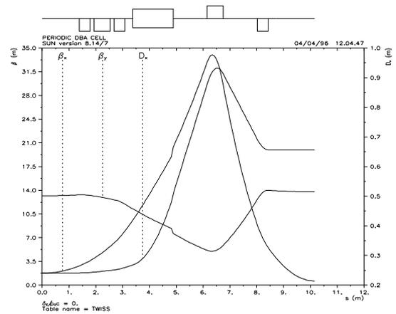
Figure 4: Lattice functions for DBA arc half cell in high emittance mode ( $\nu_x^c=5/6$ ,  $\nu_y^c=1/3$ ).
