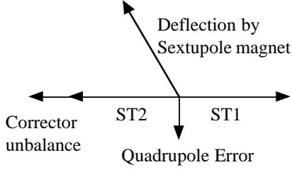
Figure 1: deflection by a sextupole magnet can be separated from strength unbalance of corrector magnets using phase information of betatron oscillation in a leakage orbit
