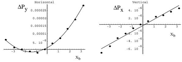
Figure 2: Deflection angle (radian) at sextupole magnet as a function of a bump orbit at sextupole magnet (mm). Results of fitting by quadratic and linear functions are also shown as solid curves.
