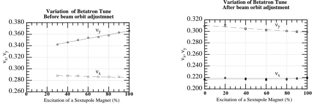
Figure 3: These figures shows betatron tune variation as a function of excitation of sextupole magnets. The left figure shows the result of measurement before beam orbit adjustment. The right figure shows the tune variation after beam orbit adjustment.
