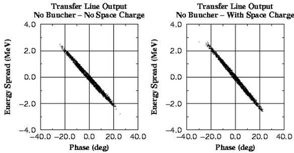
Fig. 2 Longitudinal phase space projections at the end of the ESS transfer line without a bunch rotator
