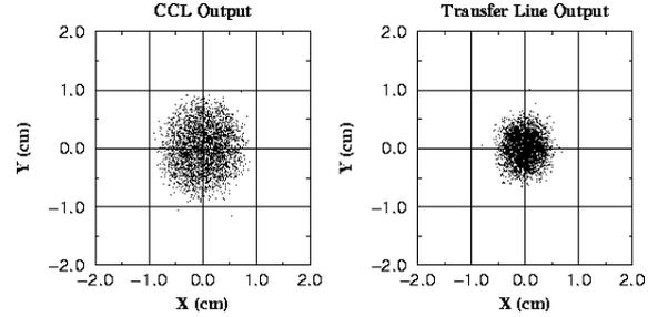
Fig. 3 Radial phase space projections at the beginning and the end of ESS transfer line. A bunch rotator is included.
