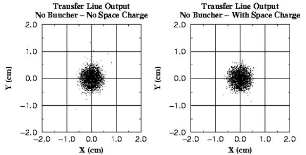
Fig. 4 Radial phase space projections at the end of the ESS transfer line. No bunch rotator is included.
