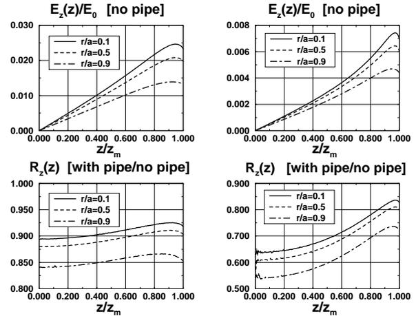
Fig. 6 The axial fields in free space (top) and the field ratios (bottom). Left column corresponds to 4 cm half bunch length and the right one to 10 cm half bunch length
