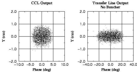
Fig. 5 Real space projections for full current at the beginning and the end of the ESS transfer line without a bunch rotator.
