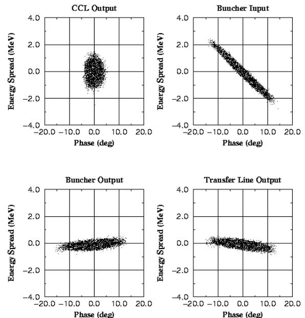
Fig. 1 Longitudinal phase space projections along the 130 m long ESS transfer line. A bunch rotator is located at 70 m.
