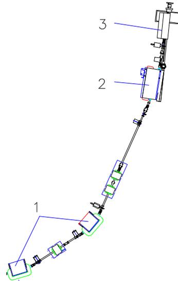
Fig. 3 Top view of transport line in the ring level with  $33^\circ$  dipole (1), the thick septum (2) and thin septum (3)
