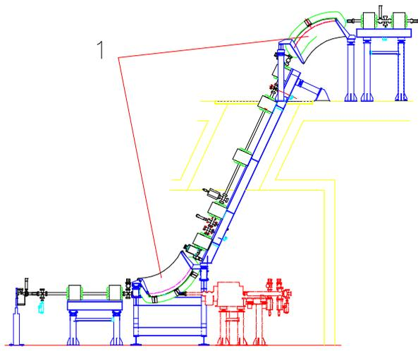
Fig. 2 Transition of under ground level and ring level, with  $65^\circ$  dipole (1) for deflection
