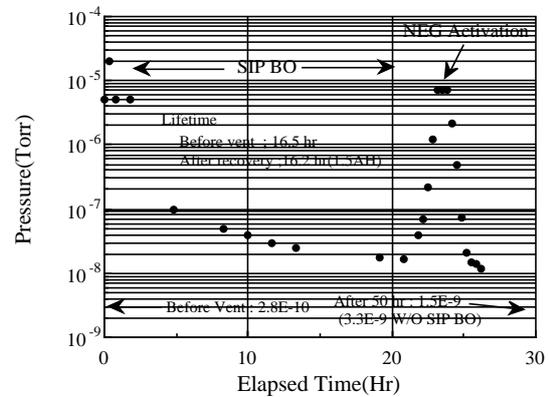
Figure 4: Pump down after air exposure
