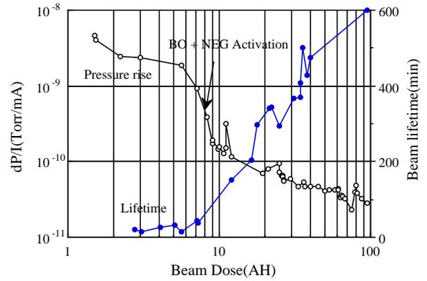
Figure 3: Beam lifetime as a function of beam dose. Data obtained with 100mA stored beam.
