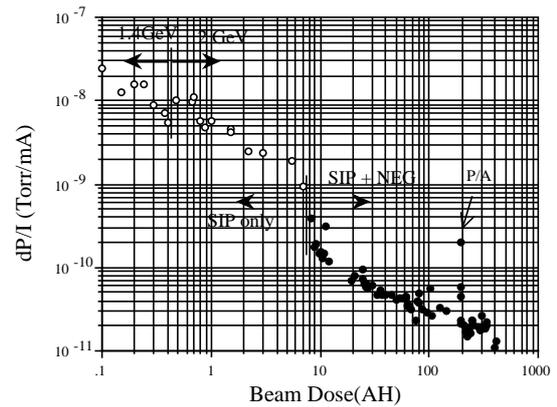
Figure 1: Reduction of pressure rise with respect to the accumulated beam dose. The arrow marked P/A points to photon absorber replacement.
