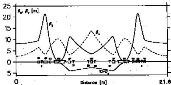
Figure 1. Theoretical Beta Functions in one Achromat
