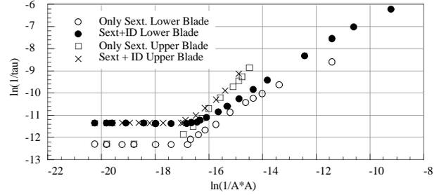
Figure 4. Vertical dynamic aperture measurement at 1.0 GeV with and without the insertion devices.
