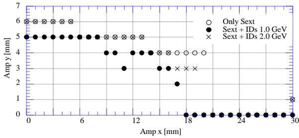
Figure 7. Results of tracking with and without insertion devices at 1.0 and 2.0 GeV.
