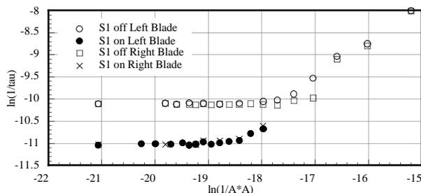
Figure 3. Horizontal dynamic aperture with and without the harmonic sextupole.
