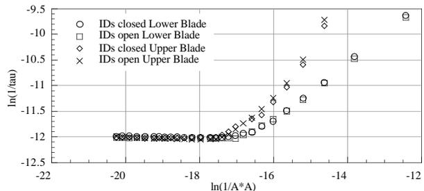
Figure 6. Dynamic aperture measurement with and without the insertion devices at 2.0 GeV.
