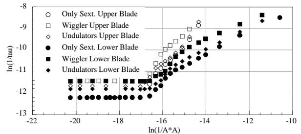
Figure 5. Comparison of dynamic aperture measurements to investigate the relative effects of the insertion devices.
