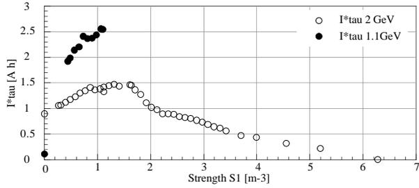
Figure 2. The beam current x lifetime as a function of the harmonic sextupole's strength.
