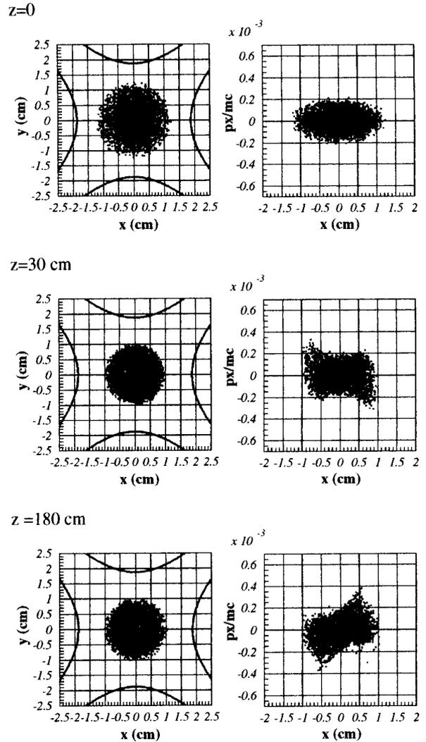
Fig. 1. Emittance growth of the 150keV, 100mA,  $015\pi$ cm mrad proton beam in a uniform four vanes quadrupole line with field gradient  $50\text{kV/cm}^2$  and frequency 270MHz.
