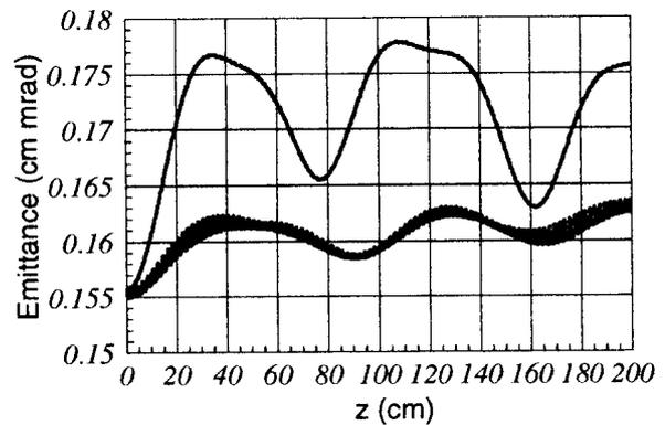
Fig. 3. Beam emittance growth in a four vane structure with pure quadrupole field (up) and in quadrupole field with duodecapole component (bottom).
