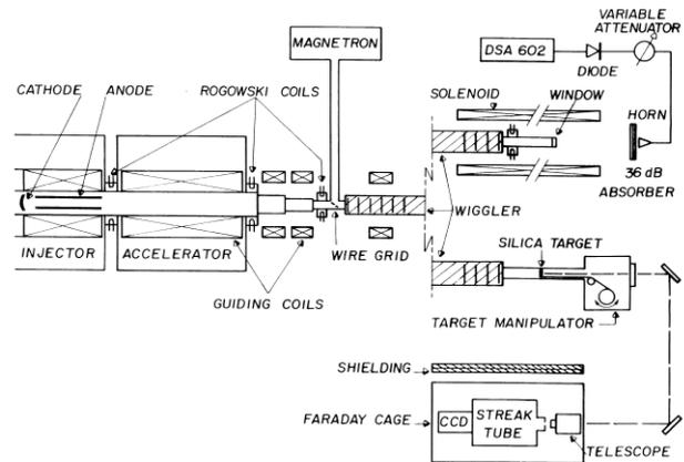
Figure: 1 Free Electron Laser (upper) and bunching measurement (lower) set-ups
