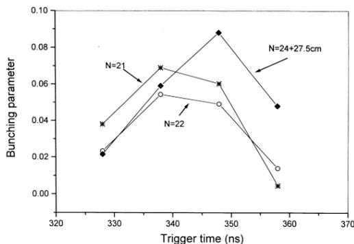
Figure 3 : Experimental bunching parameter at different time slices within the electron beam for three axial positions
