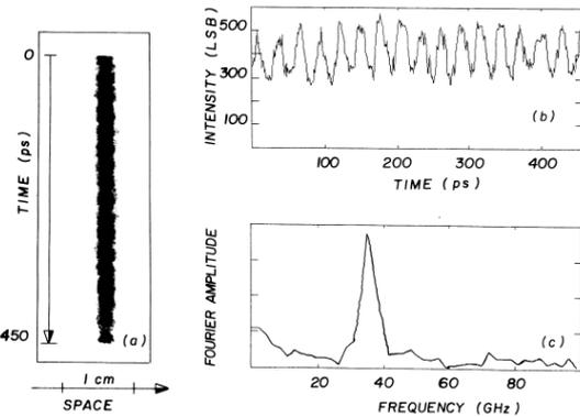
Figure 2 : Example of optical bunching measurement for a sweep speed of 25 ps/mm at a position 27.5 cm after the wiggler exit: (a) streak camera recording; (b) digitized intensity of (a) plotted vs time; (c) frequency spectrum of (b).
