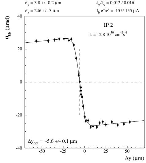
Figure 1: Beam-beam deflection scan for a beam energy of 65.1 GeV.  $\theta_{bb}$  is shown as a function of the electrostatic separator bump amplitude  $\Delta y$ . The systematic offset  $\theta_0$  is already subtracted from the data. The line is the result of the fit. The luminosity  $L$  and the beam-beam tune shifts  $\xi_x$  and  $\xi_y$  have been calculated from the fitted beam sizes and the bunch currents  $I_b$ .  $\Delta y_{\text{opt}}$  is the optimum separator setting.
