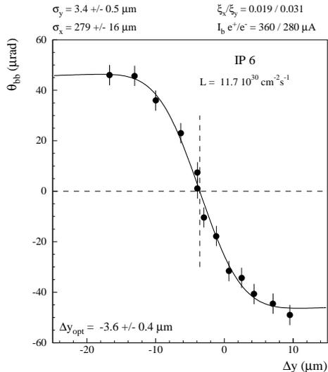
Figure 2: Beam-beam deflection scan performed at a beam energy of 68.1 GeV. The bunch currents are more than twice as large as for the scan shown in Figure 1.
