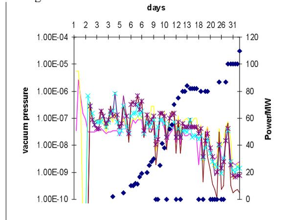
**Figure 2:** Peak Power Processing of a 5.2 meter section as a function of time. The pressure inside the section and the peak power are given in the same plot.
