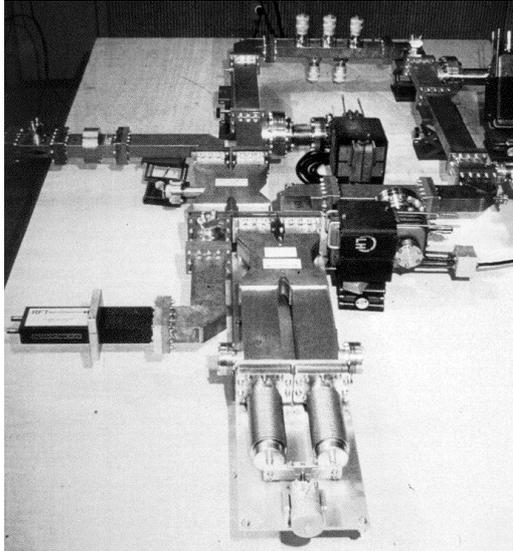
**Figure 1:** The travelling wave resonator, assembled from a closed waveguide, and coupled to a power source via a 10 dB coupler.
