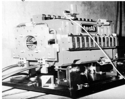
**Figure 5:** The ground motion detector with the quadrupole, the piezo driven feedback and the concrete support. The aluminum support for the coil can be seen in front.
