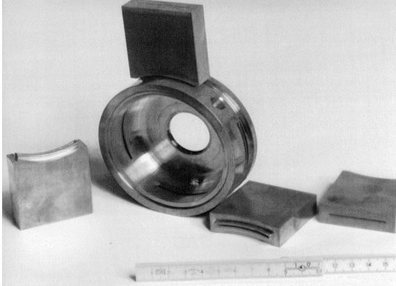
**Figure 4:** Two higher order mode couplers are integrated in the accelerating structure to couple out and measure the beam induced power in the dipole modes.
