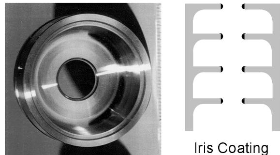
**Figure 3:** Picture of the iris coating to introduce losses for the  $\text{HEM}_{11}$  mode with only little effect on the accelerating field.
