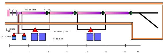
**Figure 6:** A sketch of the S-Band test facility layout with the injector, two modules similar to those used in a Linear Collider and the beam diagnostic station.
