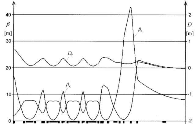
Figure 4: Optical functions of one quadrant of the DELTA low emittance optics.
