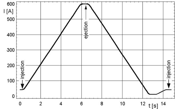
Figure 3: Ramping curve of the booster.
