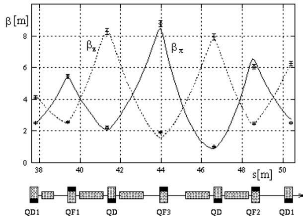
Figure 2: Optics of one quadrant of the booster. The lines are the calculated functions and the points are measured.
