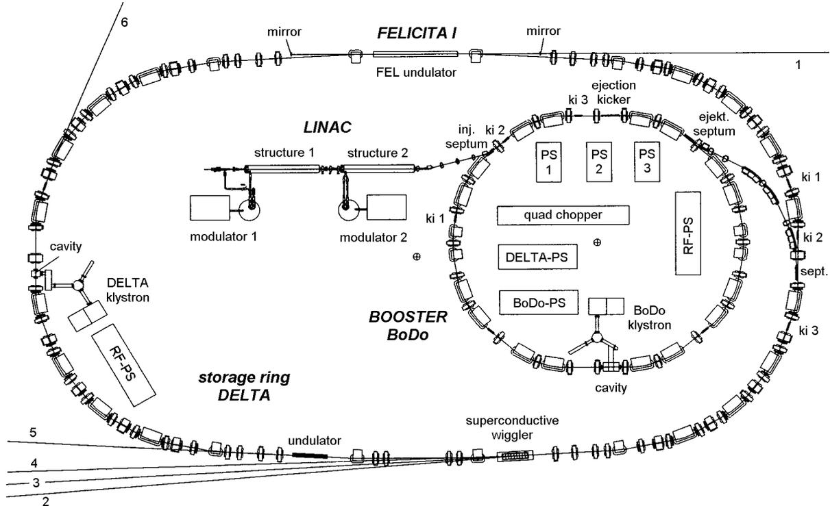
Figure 1: The electron storage ring facility DELTA with the assembled and planned experiments and beamlines. The electrons are provided by a 100 MeV linac and accelerated in a booster to the maximum operation energy of the storage ring of 1.5 GeV.
