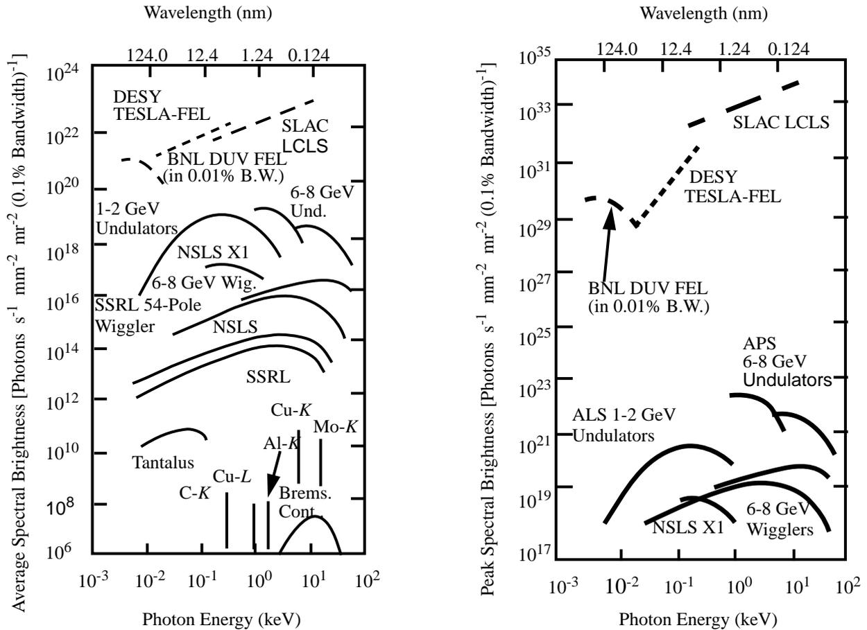
Figure 1: Comparison of average and peak spectral brightness for existing and proposed light sources
