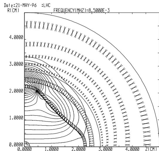
Figure 2: The field map of the field penetration between copper coating stripes.
