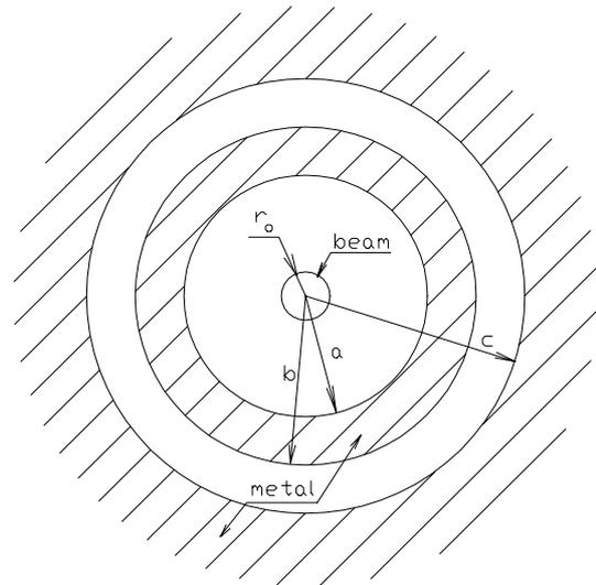
Figure 1: Cross section of the round multilayer tube.
