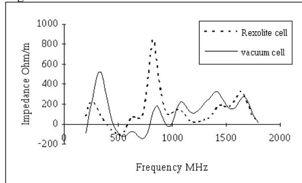
Figure 4: transverse impedance measurement: a:Rexolite technology cell; b:vacuum technology cell
