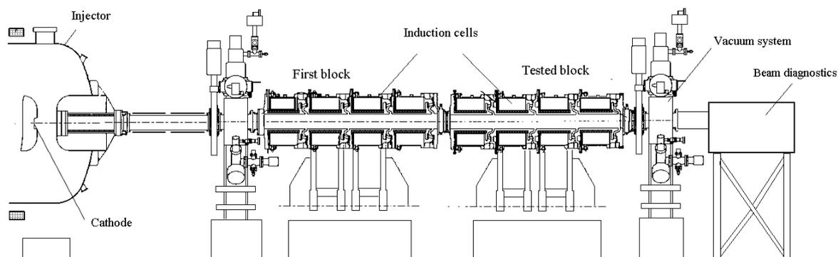
Figure 1: PIVAIR set-up with 8 induction cells
