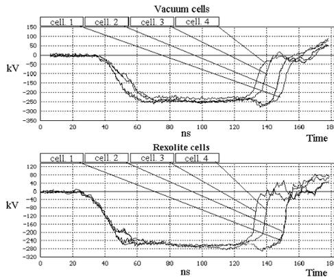
Figure 3: HV pulse measurement on 4 cells for vacuum technology and Rexolite technology
