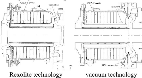
Figure 2: Design of the induction cells.
