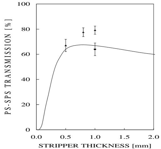
Figure 5: Estimate of PS-SPS transmission vs. stripper thickness (solid line). The measured transmission for the 1 mm thick stripper (square) and the measured stripping efficiencies multiplied by  $\eta$  for the 0.5, 0.8 and 1 mm thick strippers (triangles) are also shown.
