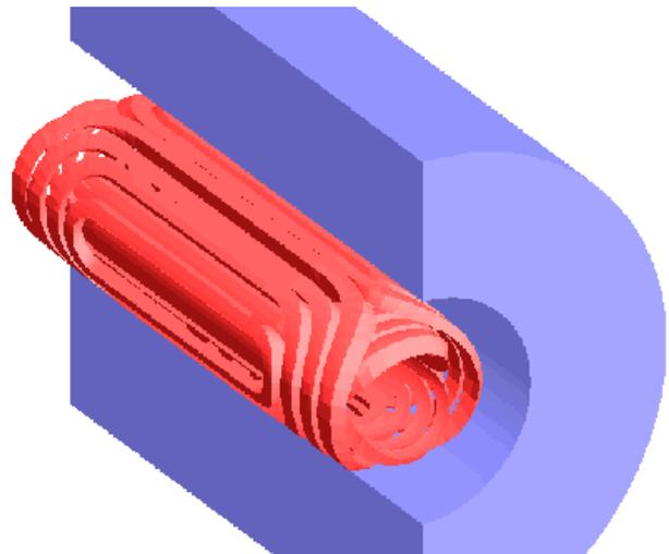
Figure : 3. MCBX-magnet Opera-3D<sup>®</sup> model. Only the return ends modelled for simplicity.
