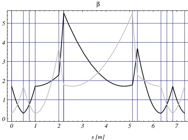
Figure 2  $\beta$ -plots in a phase-shifter.
