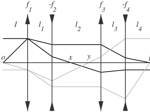
Figure: 1 Particle trajectories in a thin lens telescope.
