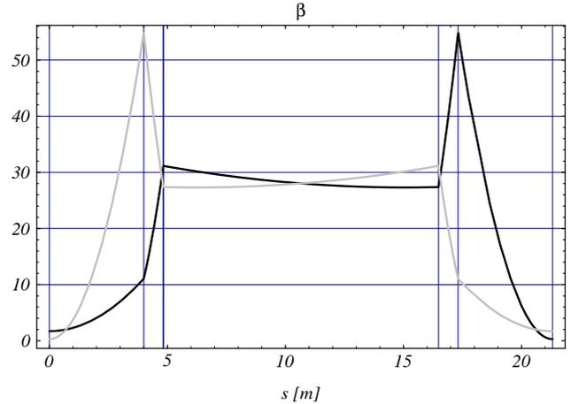
Figure 4  $\beta$ -plots in a high beta insertion
