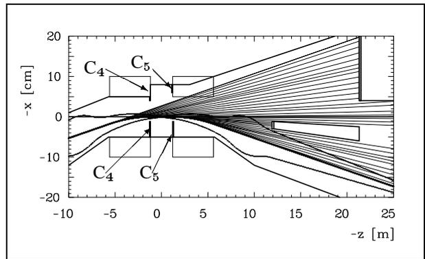
Figure 6: Synchrotron radiation fan from air-coil separator.  $\gamma$ -flux actually striking absorber protecting the septum is  $2 \times 10^{17}/s$ . Collimators  $C_4$ ,  $C_5$  are placed inside detector to catch backscatter.
