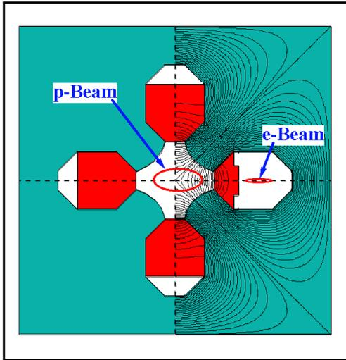
Figure 5: Beam separation schematic at current septum quadrupole.
