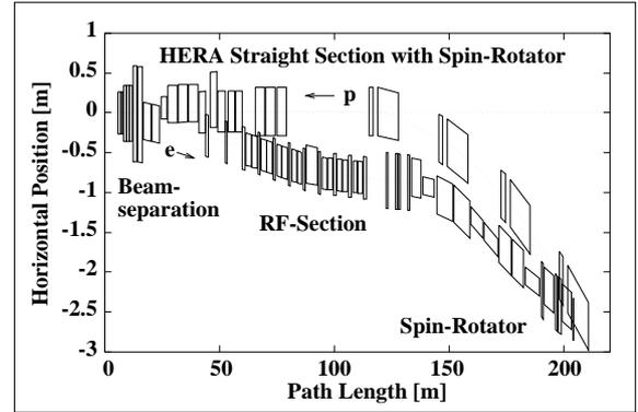
Figure 1: Present HERA e-p IR design layout (plan view) with spin-rotator.
