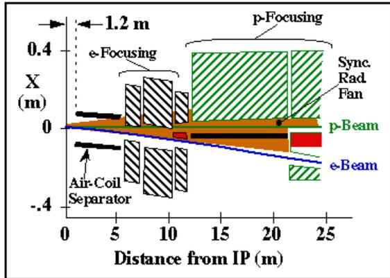
Figure 2: Example of early separation via weak air-coil dipole integrated inside detector. Separate p-focusing starts at 12.5 m using special quadrupoles.
