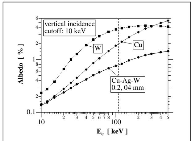
Figure 7: Comparison of backscattered synchrotron radiation albedo for coated and uncoated tungsten absorber.
