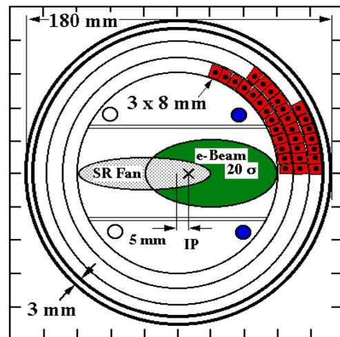
Figure 3: Air-coil separator magnet with  $B = 0.187$  T ( $E_{crit} = 109$  keV).
