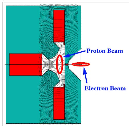
Figure 4: Beam separation schematic at magnetic septum quadrupole with  $R_{pole} = 40$  mm and 20 T/m gradient.
