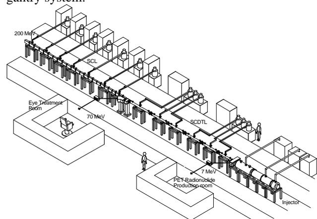
Figure 1. Layout of the TOP - ISS proton linac
