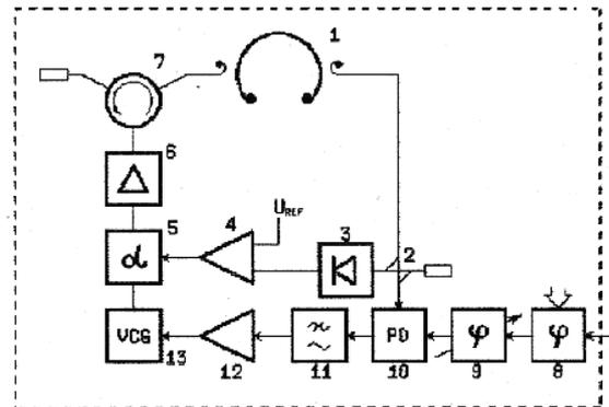
Fig.3 The chopper RF feed system.
