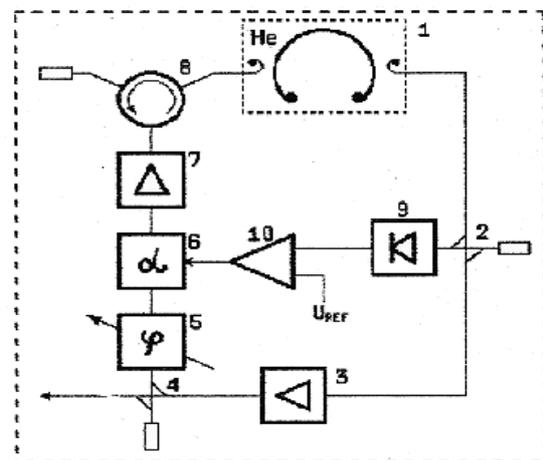
Fig. 2. The SCC RF feed subsystem functional scheme.
