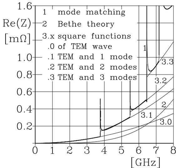
Figure 6: comparison of real part of impedance for a square hole with 4 mm edge length versus frequency calculated by mode matching (1); compared with the square behaviour (3.x), (3.0) including TEM wave, (3.1) including also 1 waveguide mode, (3.2) 2 modes, (3.3) 3 modes; and by Bethe hole coupling (2);  $b=16\text{mm}$ ,  $d=5\text{mm}$
