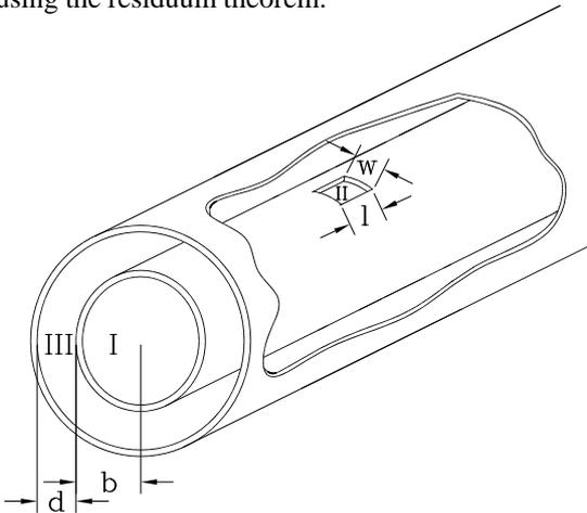
Figure 1: scetch of the liner structure
