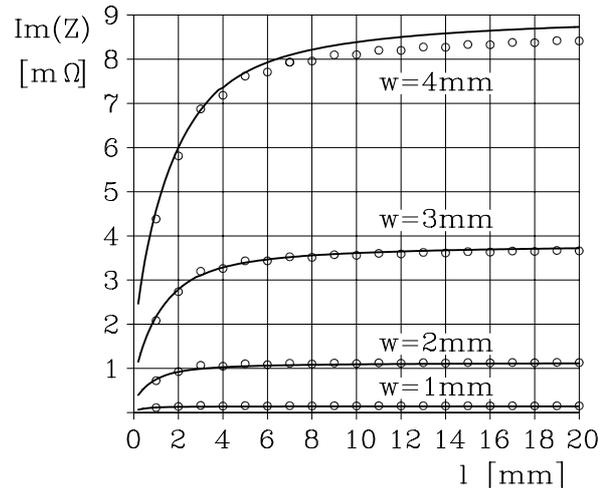
Figure 2: comparison of imaginary part of impedance for slots with the width  $w$  and the length  $l$  at 1 GHz calculated by Bethe hole coupling (solid line) and by mode matching (dots);  $b=16\text{mm}$ ,  $d=5\text{mm}$
