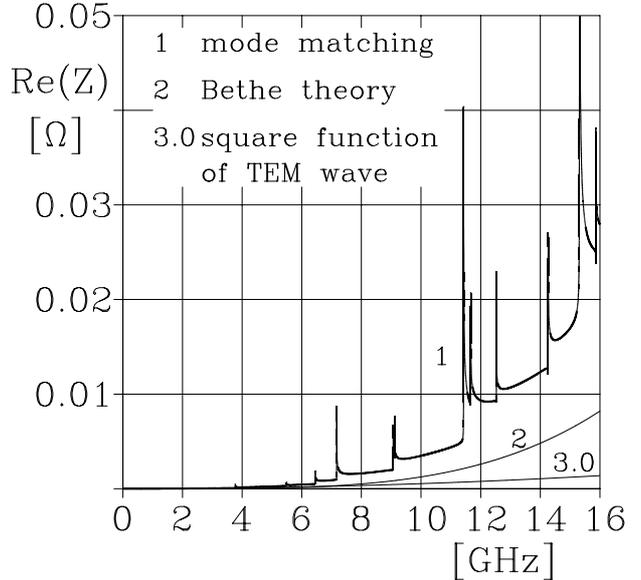
Figure 5: comparison of real part of impedance for a square hole with 4 mm edge length versus frequency calculated by mode matching (1); compared with the square behaviour for TEM wave (3.0); and by Bethe hole coupling (2);  $b=16\text{mm}$ ,  $d=5\text{mm}$
