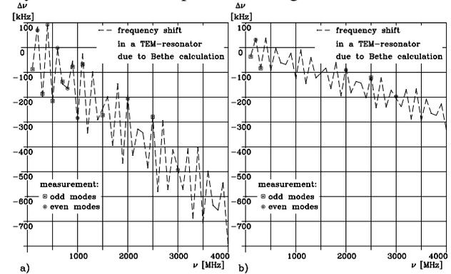
Figure 9: frequency shift versus resonance frequency of the TEM-line for 200 holes with a) 4mm diameter and b) 3mm diameter, calculation (dashed line) and measurement (points)
