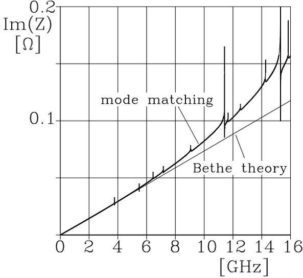
Figure 3: comparison of imaginary part of impedance for a square hole with 4 mm edge length versus frequency calculated by mode matching (thick line) and by Bethe hole coupling (thin line);  $b=16\text{mm}$ ,  $d=5\text{mm}$
