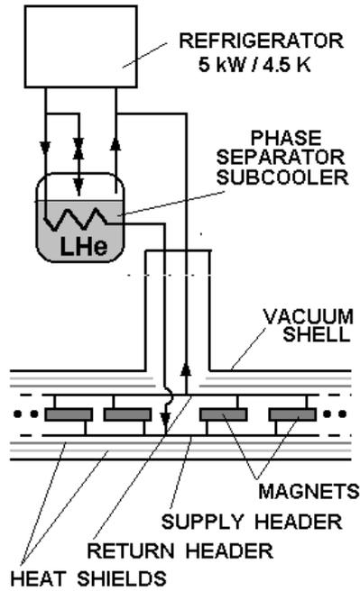
Figure 3: A possible unit of 2×5 km long of cryomagnetic system for a multi-TeV range accelerator
