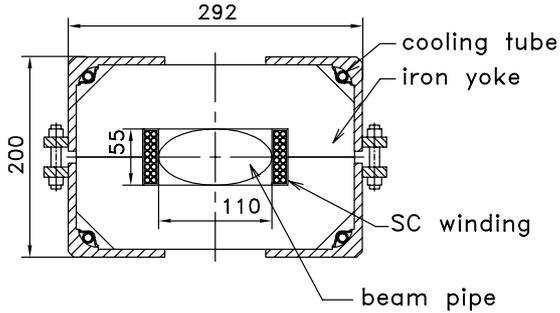
Figure 2: Cross-section of the Nuclotron dipole
