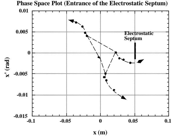
Fig. 5. Amplitude Increase for Larger Emittance Beam (at the Electrostatic Septum for Extraction).
