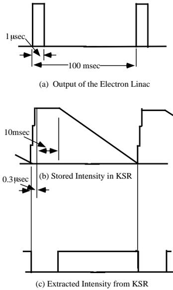
Fig. 2 Scheme of KSR Stretcher Mode.
