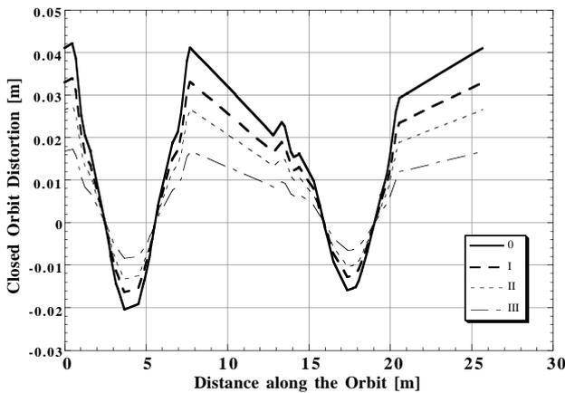
Fig. 3 Closed Orbit Distortion caused by a Perturbator.
