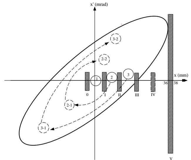
Fig. 4 Phase space plot of the injected beam at the exit of the inflector. The shaded areas show the septum positions during several turns after the start of injection. The number in the circle indicates the injection turn number. The number after hyphen indicates the circulation number of the injected beam.
