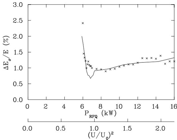
Figure 5: Comparison between the calculated (solid line) and measured (dots) energy spread  $\Delta E/E$  to determine the shunt impedance
