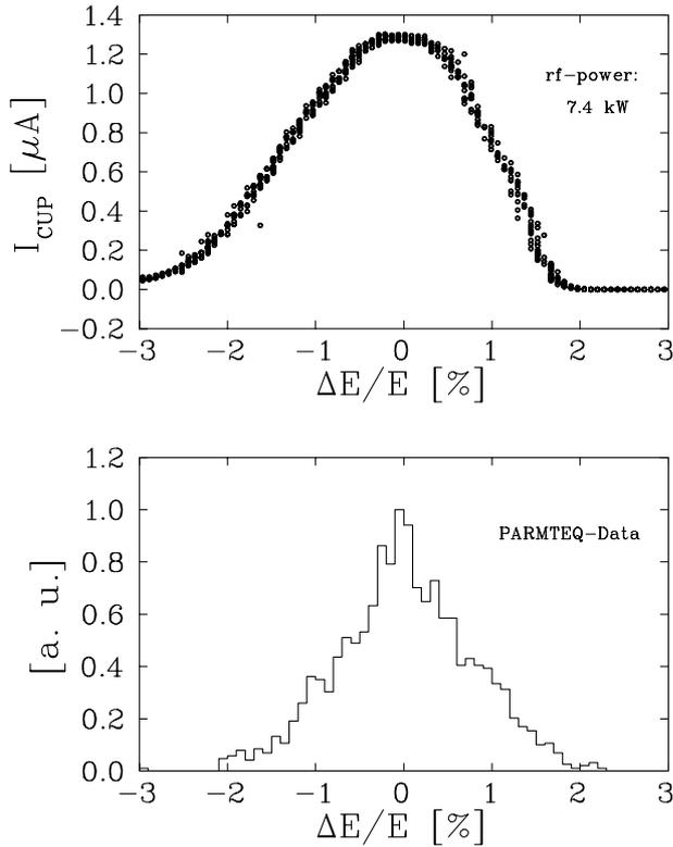
Figure 4: Calculated (line) and measured (dots) energy distribution at an electrode voltage of 15.8 kV
