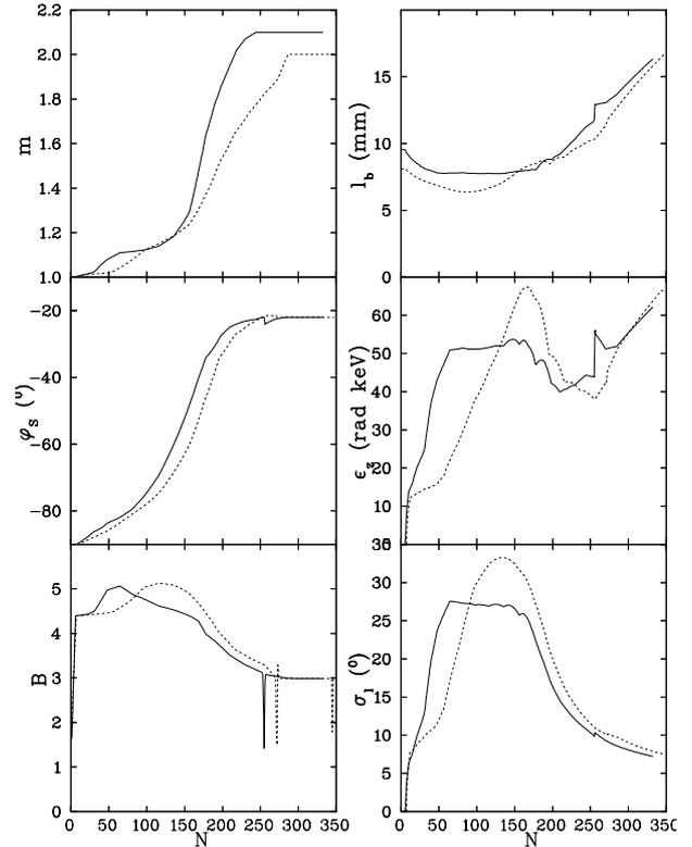
Figure 6: Parameters of the re-designed electrodes: dashed line=old design, solid line=new design.  $m$ =modulation,  $\phi$ =phase,  $B$ =focussing parameter,  $l_b$ =bunchlength,  $\epsilon$ =emittance and  $\sigma$ =phase advance
