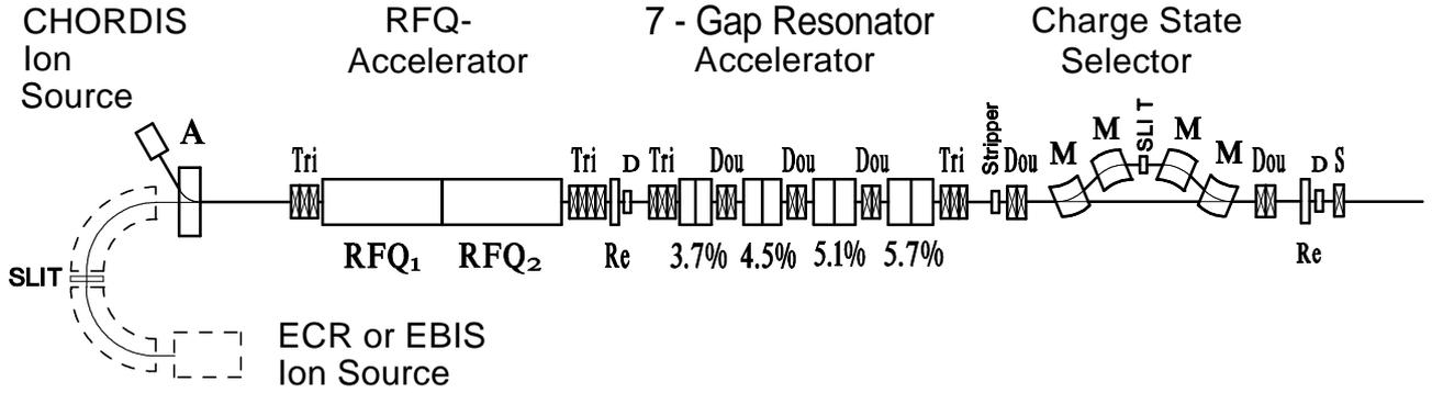
Figure 1: Schematic layout of the new high current injector. A, M, S, Dou, Tri: magn. dipoles and lenses, Re: rebuncher, D: beam diagnostic. The ion source for highly charged ions (ECR or EBIS) and the charge state selector are planned for the second construction phase. The ion source will then be located one floor below.
