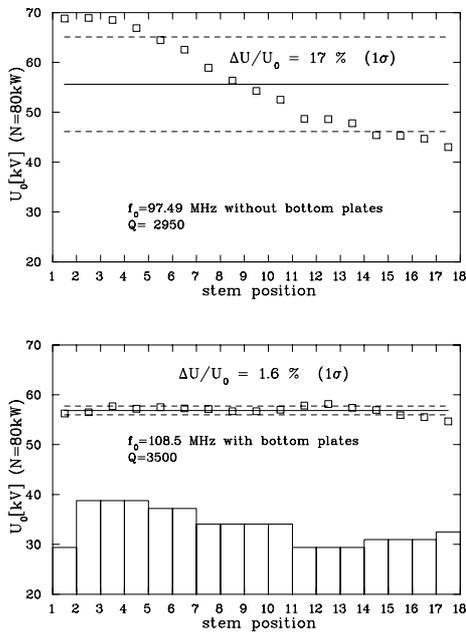
Figure 2: Voltage distribution and eigenfrequency of the RFQ-resonator with and without tuning plates
