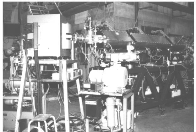
Figure 3: Left side: analyzing magnet and diagnostics. Right side: the RFQ-resonator
