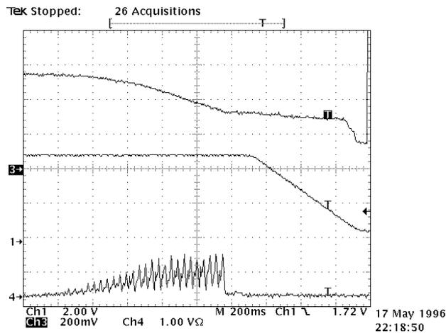
Figure 4. DCCT signal (upper) and current pattern (middle) with the partially extracted beam signal(lower).
