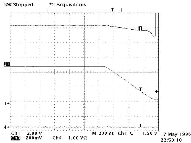
Figure 3. DCCT signal (upper) with current pattern (lower) at the deceleration. Horizontal scale is 0.2 sec/div..
