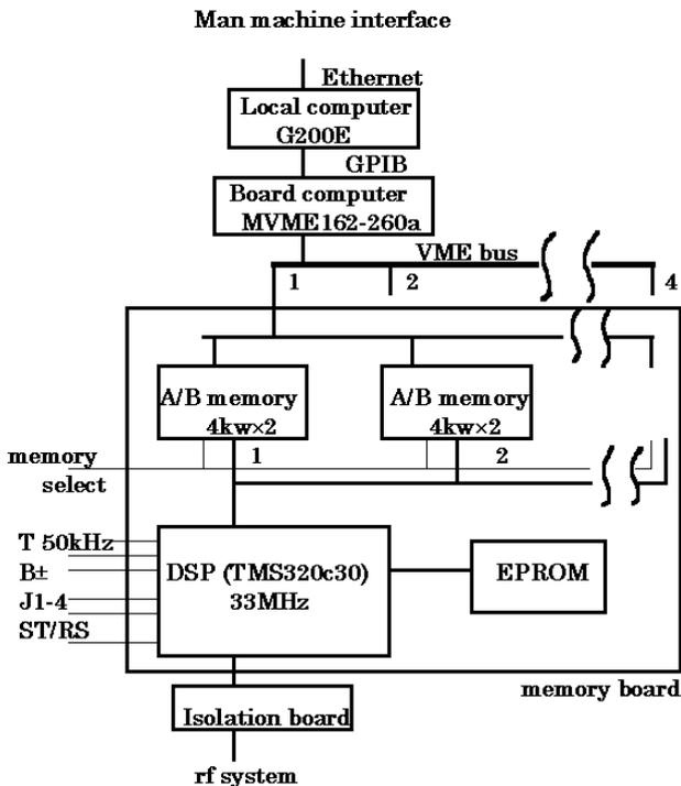
Figure 1. The new pattern memory with the interface computers.
