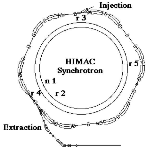
Figure 4. Layout of the HIMAC synchrotron and the monitors of the radiation level.
