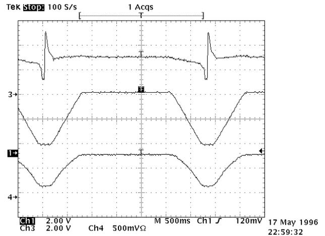
Figure 2. The beam signal with the deceleration (upper signal). The middle and lower signals are the current of the magnet and the acceleration frequency, respectively. Horizontal scale is 0.5sec/div.
