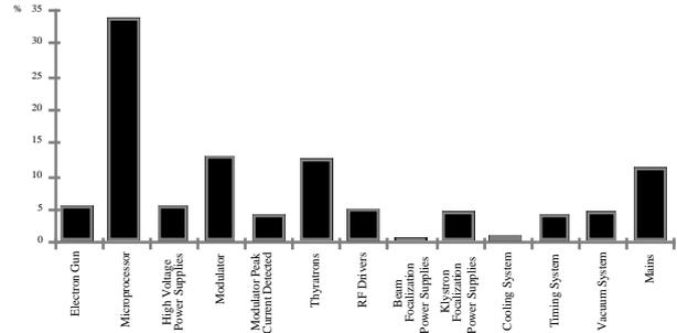
Figure: 1 Linac subsystems downtime statistics (RUN 12 - RUN 30) in percentage of the total Linac downtime.
