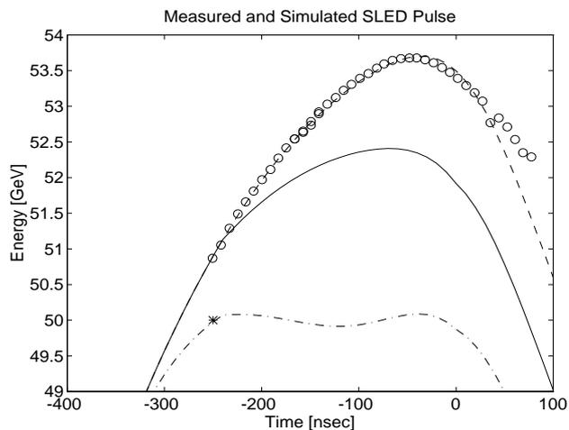
Figure: 4 Beam energy gains simulated and measured
