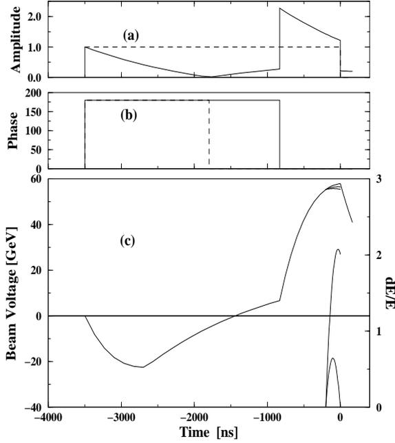
Figure: 1 SLED input (dashed) and output (solid) a) Amplitude b) Phase c) Beam voltage, loaded voltage; and energy spread (lower curves).
