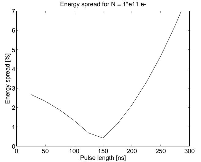
Figure: 2 Maximum energy spread versus  $t_b$  for  $10^{11} e^-$
