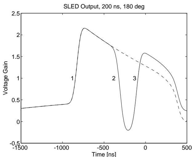
Figure: 3 RF amplitudes with 1 and 3 phase inversions
