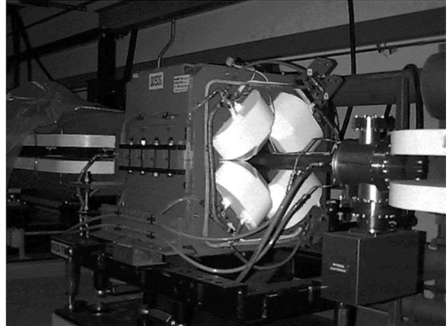
Figure 1. Quadrupole raft installed in the PEP Tunnel
