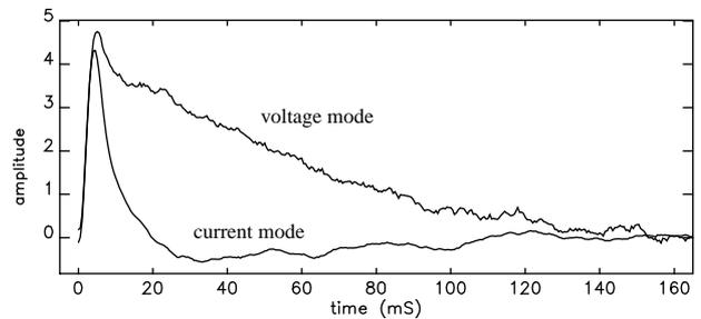
Figure 7: Impulse Response of Wiener Filter Forward Models
