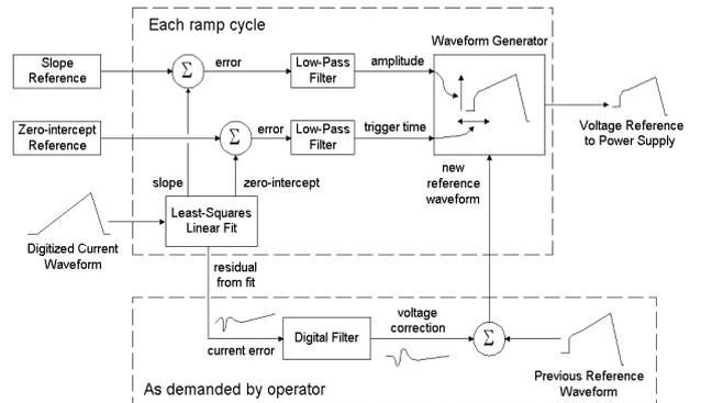
Figure 1: Control Scheme for Voltage Mode
