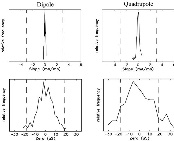
Figure 2: Deviations from Nominal Values over 24 Hours (dotted lines indicate target worst-case errors)
