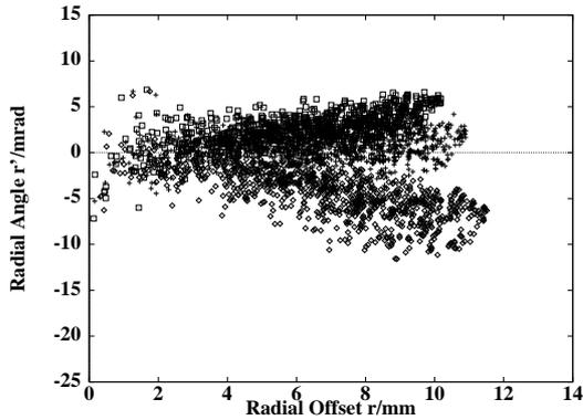
Figure 7: Transverse phase space of the first, middle and last bunch behind the solenoid (New design),  $E=100$  MV/m.
