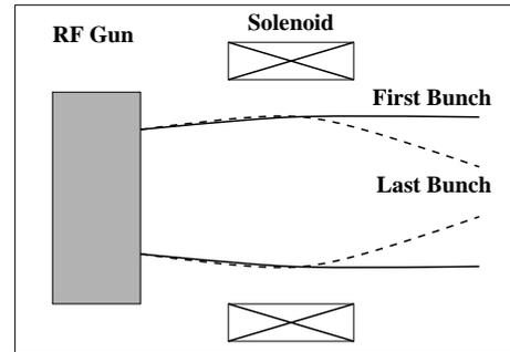
Figure 5: Schematic beam trajectories showing the chromatic effects in the solenoid caused by the beam loading.
