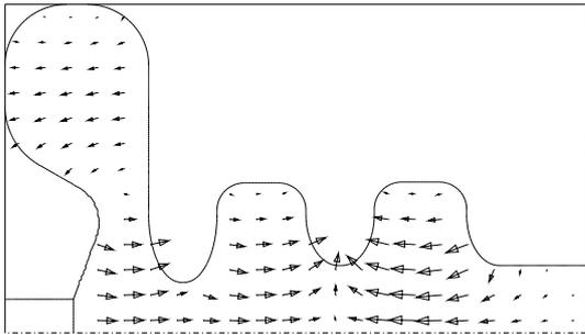
Figure 3: Secondary mode ( $f=2990.5$  MHz) involved in beam loading.
