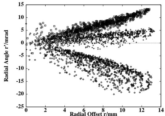
Figure 1: Transverse phase space plot of the first, middle and last bunch behind the solenoid (3  $\text{TM}_{01}$  cells).
