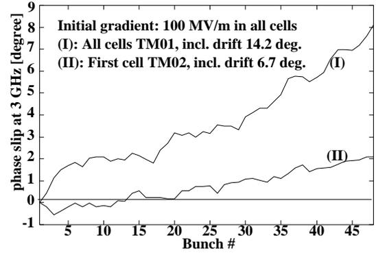
Figure 4: Phase slip, (I): all cells  $TM_{01}$ , (II): first cell  $TM_{02}$ .
