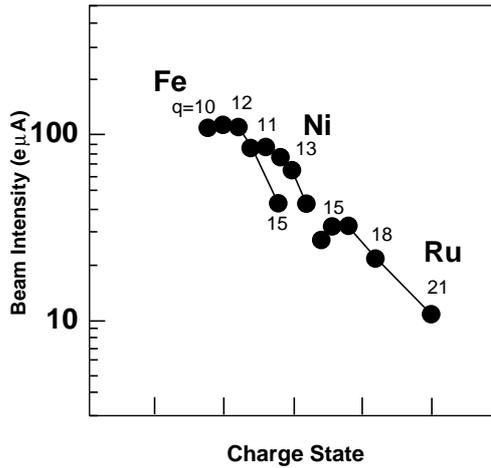
Fig.4. Charge state distributions of Fe, NI, and Ru ions using MIVOC method.
