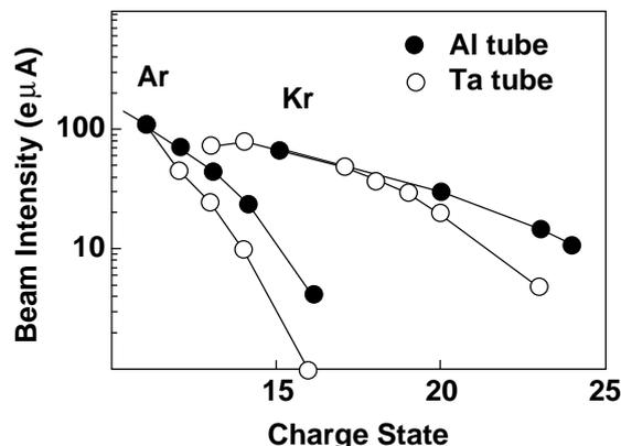
Fig.3. Charge state distribution of Ar and Kr ions. Open and closed circles represent the results obtained with a Ta and Al tube, respectively.
