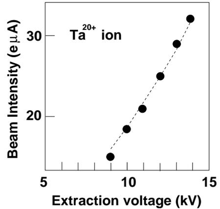
Fig. 6. Beam intensity of Ta<sup>20+</sup> as a function of extraction voltage.
