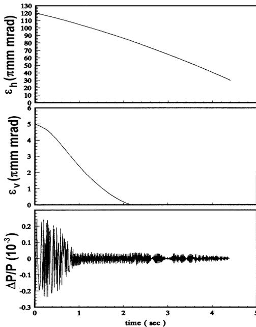
Fig.2 The time evolution of beam emittance and momentum spread with time.
