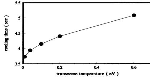
Fig.4 The transverse cooling time as a function of the electron beam transverse temperature. In these calculations,  $f_n = 90\%$ ,  $D_h = 0m$ .
