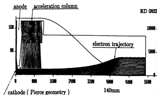
Fig.1 Computer generated plot of electron gun, acceleration column and expanded electron beam
