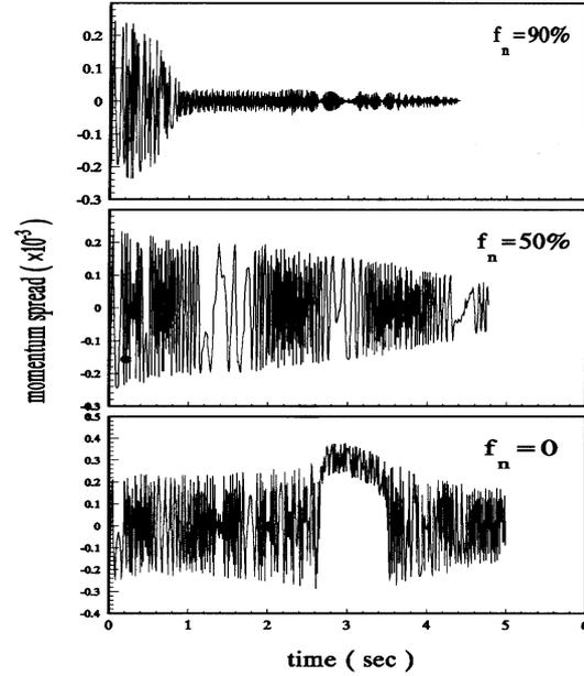
Fig.3 Longitudinal cooling resulted from the simulation for three values of neutralization factor.
