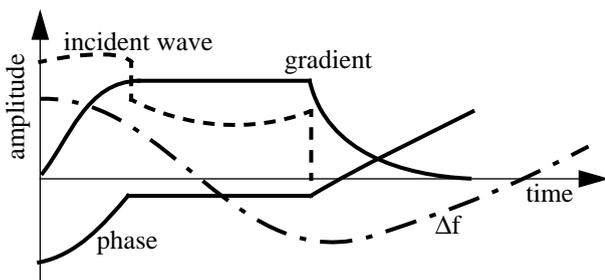
**Figure 2 :** Closed loop response. No beam. Amplitude and phase are constant during beam acceleration. The forward power is time dependent due to time varying cavity detuning.
