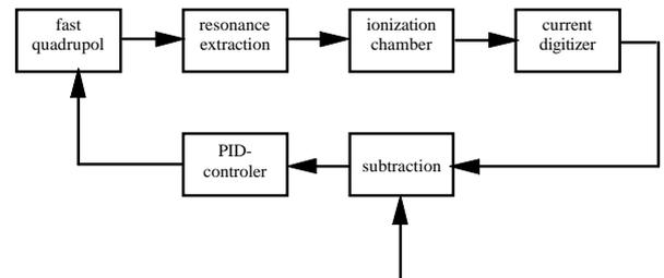
Figure 2: Schematic diagram of the feedback control system
