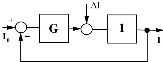
Figure 1: Simplified feedback control system.
