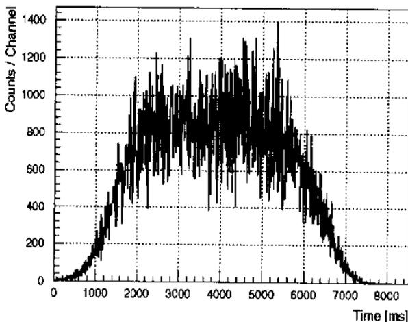
Figure 3: Slow resonance extraction without feedback.
