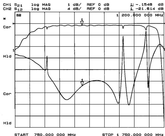
Figure 5: Custom circulator frequency response.
