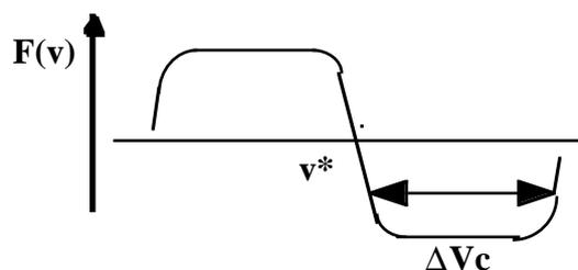
Figure 1.b Cooling force generated by two counterpropagating white-light laser beams.
