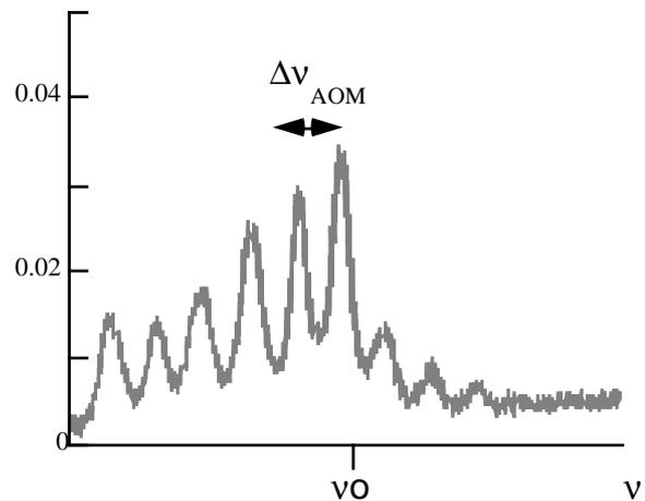
Figure 3. Fabry-Perot transmission of laser signal (arb.units) after the second AOM. The frequency of input laser is indicated by  $\nu_0$ .
