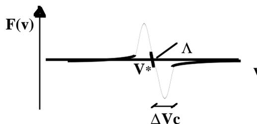
Figure 1.a Cooling force generated by two counterpropagating monochromatic laser beams.
