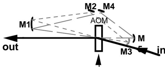
Figure 2. Sketch of the cavity configuration. The different dashed lines evidence the two intersecting rings.  $M_i$  = mirrors
