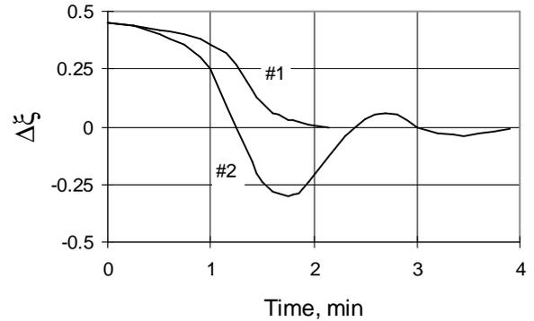
Figure 1:  $\xi(t)$ -transient in the tank #2 after repeated channel turn-on.  $\Delta\xi = \xi(t) - \xi_0$ .
