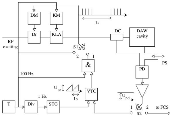
Figure 2: Block-diagram of the automatic control system for fast average RF power raising.
