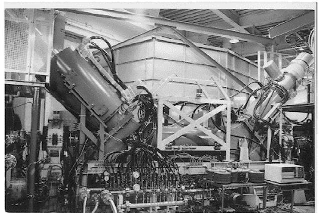
Figure 1: Photograph of the adiabatic expansion-type electron cooler with a normal-conducting magnet. The electron gun is installed in the big solenoid on the left-hand side. The length of the cooling section is 1.5 m.
