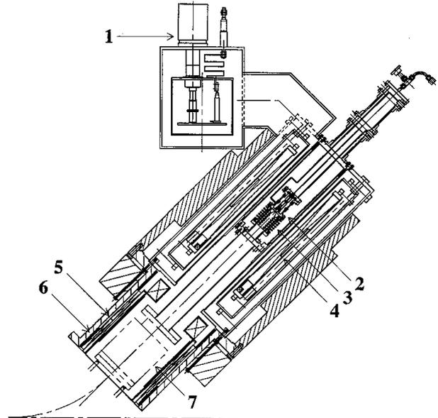
Figure 3: Layout of the electron gun region: (1) refrigerator, (2) electron gun, (3) acceleration tube, (4) superconducting solenoids, (5) normal-conducting solenoids, (6) steering coils, (7) NEG pump.
