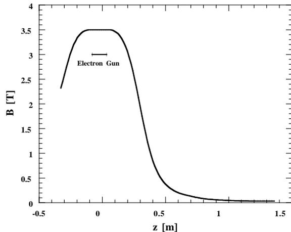
Figure 4: Calculated magnetic field produced by a superconducting solenoid followed by normal conducting solenoids.
