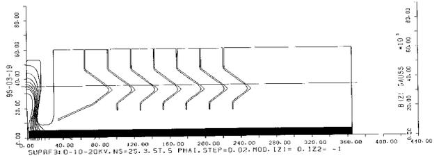
Figure 2: Calculated electron trajectories in the gun region.
