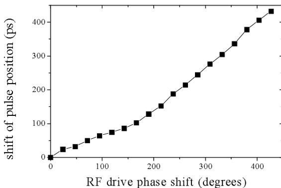
Figure 6. Control of pulse timing for operation at 2360 MHz with pulses of 50 ps duration and 100 mW average power.
