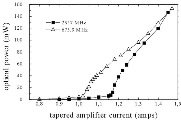
Figure 5. Light-current curve for 680 and 2360 MHz operation
