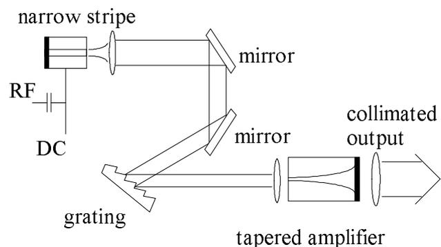
Figure 1. Schematic of Laser Cavity
